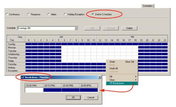
Fig. 7–5. Breakdown of a Cell into Fifteen-minute Sections.
